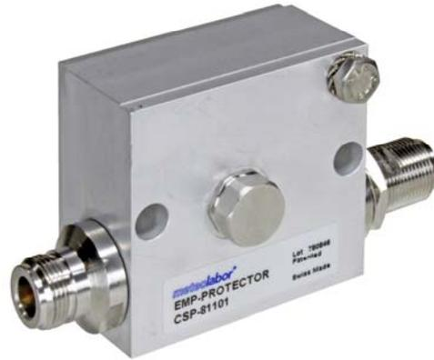
The Meteolabor® CSP series RF EMP protectors are specially designed for the protection of coaxial lines. High surge currents on the inner conductor can be handled. A unique mechanical bulkhead design offers easy feed-through installation and compact fitting into Faraday cages, shielded rooms and mechanical enclosures. Single point of entry concepts can be simply realised. This allows clear separation of unprotected and protected side.
